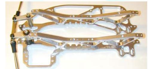
2.4. **Attach Front & Rear end:** Use the screws provided to attach the front end, M3x12 SHCS (qty. 4). The rear uses M3x12 SHCS (qty 2) and M3x 12 FHCS (qty2.)
