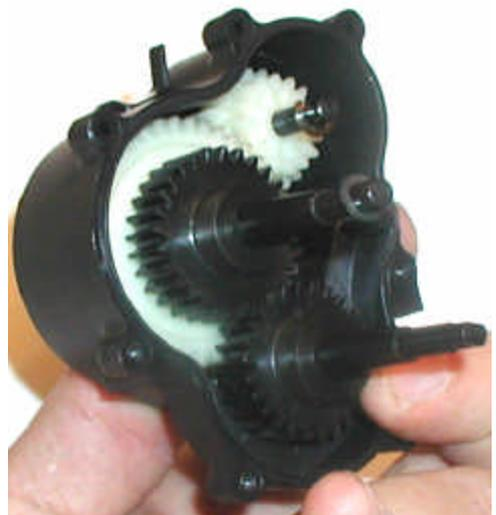
half of the transmission case and install shafts with the appropriate shims. In this order:
