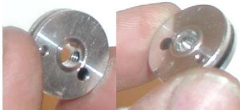
*Pro Tip: Replace that short set screw with a longer one (M4x8.) There's a lot of force on these and they can strip out the aluminum hub.*
