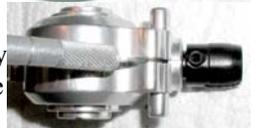
**3.2. Prepare the carrier and ring gear.** Do not install the spider gears yet. You will do this only after you have correctly set up the ring and pinion.
