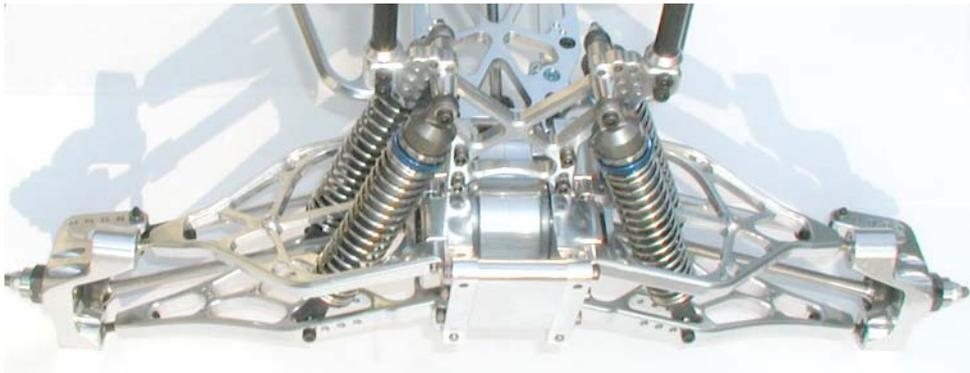
4. **Install differential in your truck** by reversing the disassembly process.
