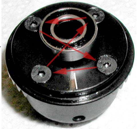
**3.3.1.3.** Gently squeeze the housing. Don't force it. You will probably see a small gap, as normally .040" of shim (four of the .010") is too much, though it's a good starting point. If a gap, go to step 4, if fully closed go to step 5.
