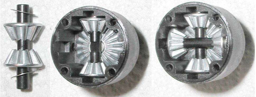
**3.4.14.** Repeat for the other one and install in the carrier such that the two shafts' flats face each other and interlock.
