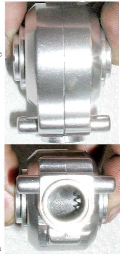
3.3.2.5. Since this is usually an interference setup, but gives you a good starting point, remove one of the .010" shims on the pinion shaft and try again. When you go to reassembly, hold the carrier in the housing perpendicular and look for a small gap between the end of the pinion and the body of the carrier. You do want a small gap here.
