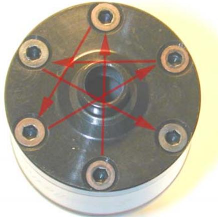
**3.2.1.** Carefully inspect the mating surfaces of the carrier and the ring gear for burrs or debris. Clean/de-burr as necessary.
