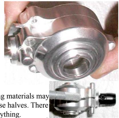
**3.2. Prepare the carrier and ring gear.** Do not install the spyder gears yet. You will do this only after you have correctly set up the ring and pinion.
