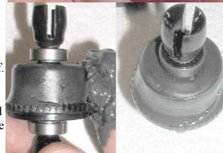
3.4.2.10. Take apart and grease. A layer of grease on the ring gear teeth is all that is necessary, putting more in does no good and only makes a mess when you need to service the differential.
