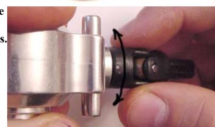
3.4.2.9. Add and tighten the case screws and check again. The final squeeze down of the screws may affect what you've done so far, in which case you'll need to re-shim the diff.
