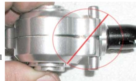
3.4.2.7. Check for free movement. It is normal for *one spot* in the rotation to be slightly tighter than the rest as no ring and pinion, no matter how precise, is perfect. You are shimming for NO tight spots w/o having excessive backlash.
