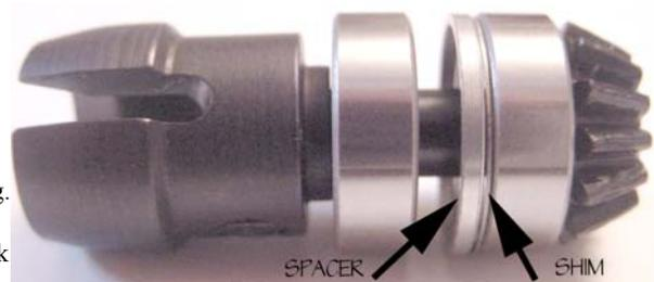
3.4.2.2. Set the pinion with it's bearings, spacer & shims down in one half of the case, then attach the pinion drive cup, then attempt to close the case.
