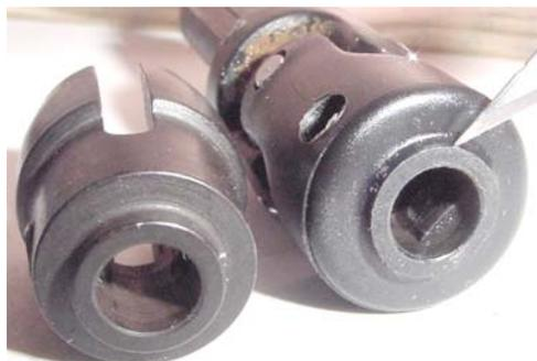
3.4.2.3. Once you have the input drive cup mounted with no pre-load on the bearing, remove the pinion set screw, apply red Loc-tite to it and reinstall into the drive cup. **TIGHTEN**
