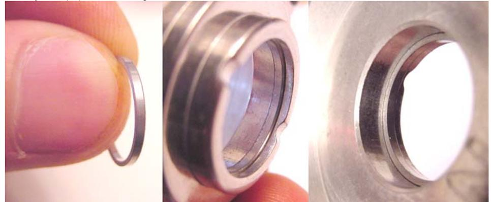
3.4.1.3. Set the ring gear down inside one of the case halves. The inside of the cases have been marked with an "N" for 'Nitro' and an "E" for 'Electric.' You will put the ring gear on the side that is correct for your application.
